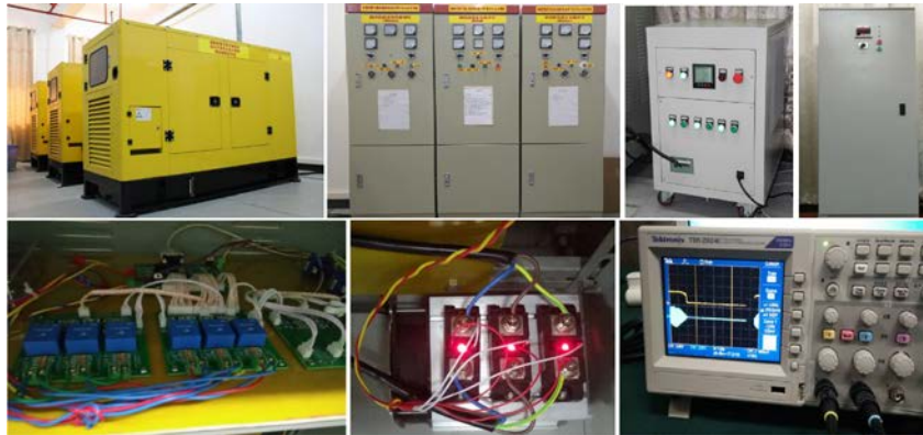
Fig.12. f/P control experiment of grid connection of voltage envelope
