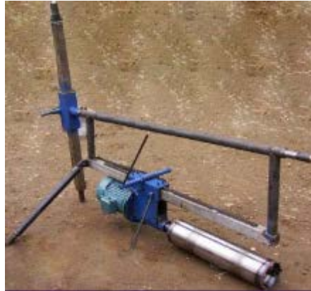
Fig. 1 Schematic diagram of water grinding and drilling equipment
