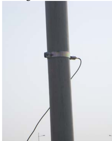
Fig.5 Arranging a Ferrule on the Rubber Sleeve
