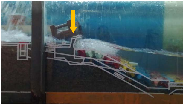
Fig.4 Measurement of Wave Overtopping volume on the top of wave wall
